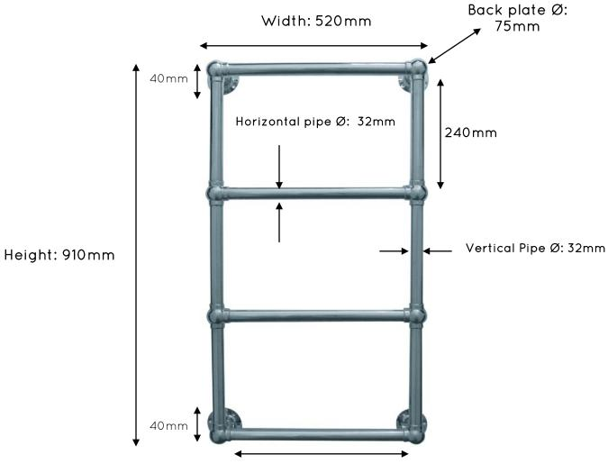
Pipe Centres: 315 mm (With solar angle valves)
